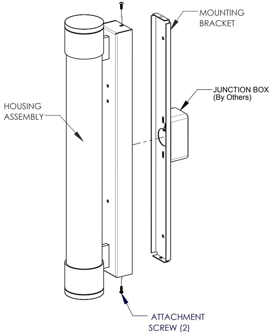
1. Fasten mounting bracket over junction box (by others) to the wall with mounting screws supplied or ones suitable for wall construction, through mounting holes.
