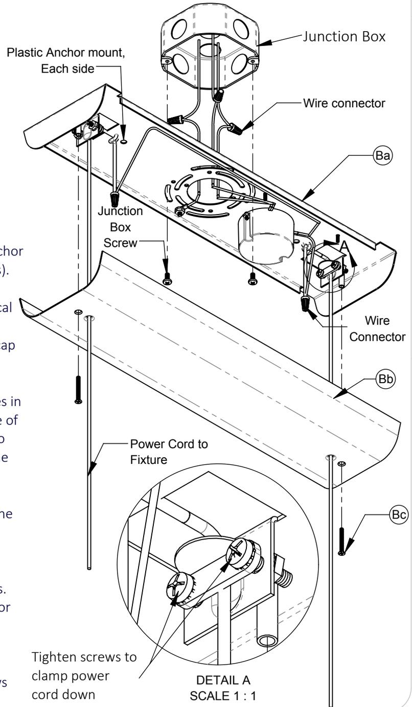
1. Remove the Cover Screws (Bc) holding onto the Cover (Bb). Save for later.
