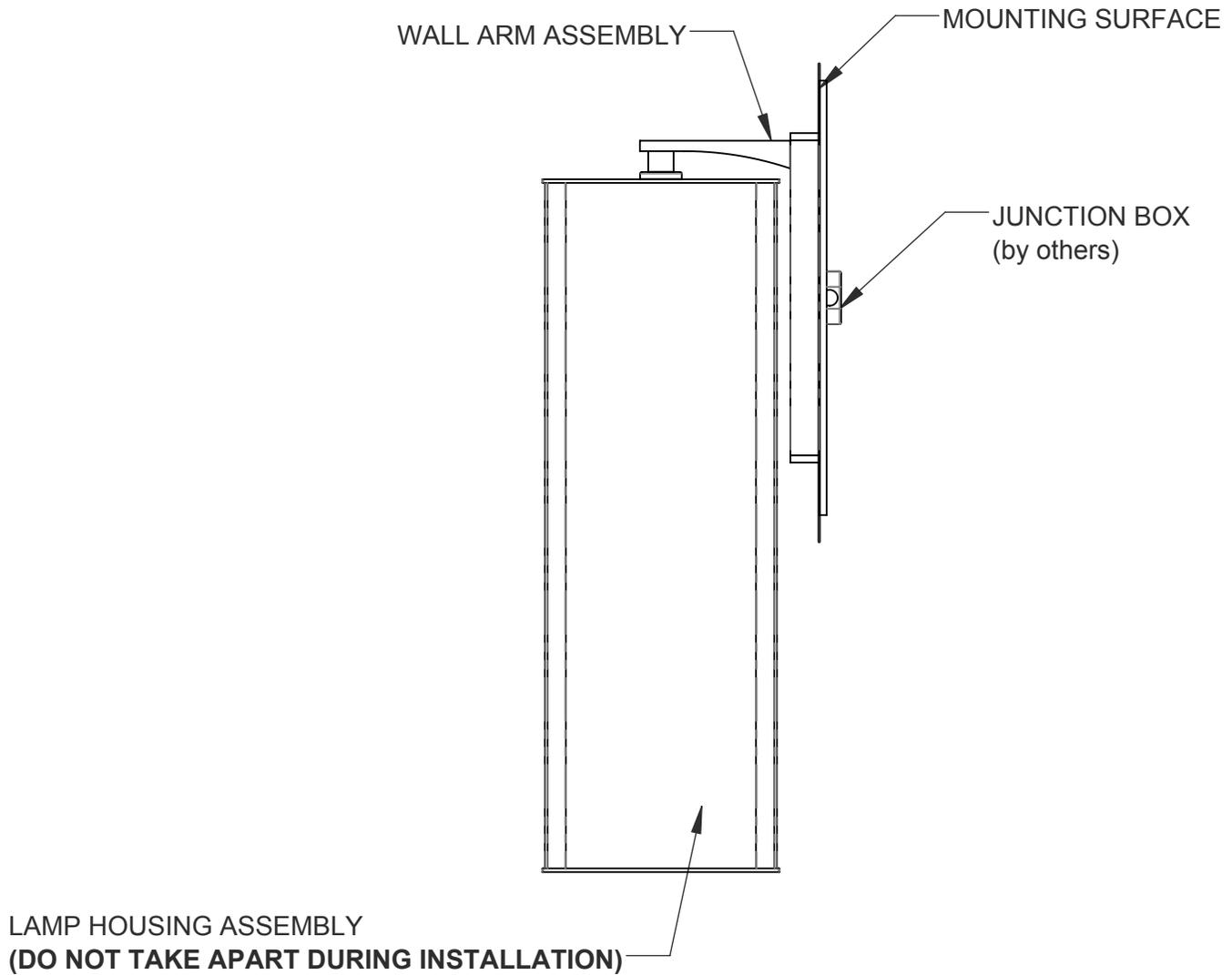
EXAMPLE OF HOW THE FINISHED PRODUCT SHOULD LOOK LIKE ONCE INSTALLED ON WALL.
