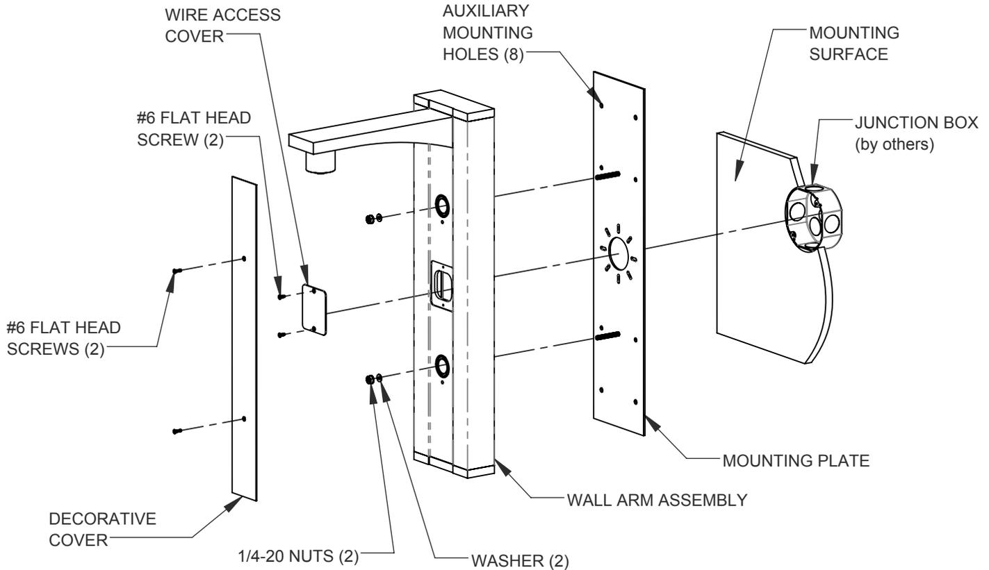
**\*NOTE:** LAMP HOUSING IS NOT SHOWN (FOR REFERENCE ONLY) TO HELP WITH INSTALLING FIXTURE TO THE WALL. REFER TO PAGE 5 FOR COMPLETE FIXTURE DETAILS.
