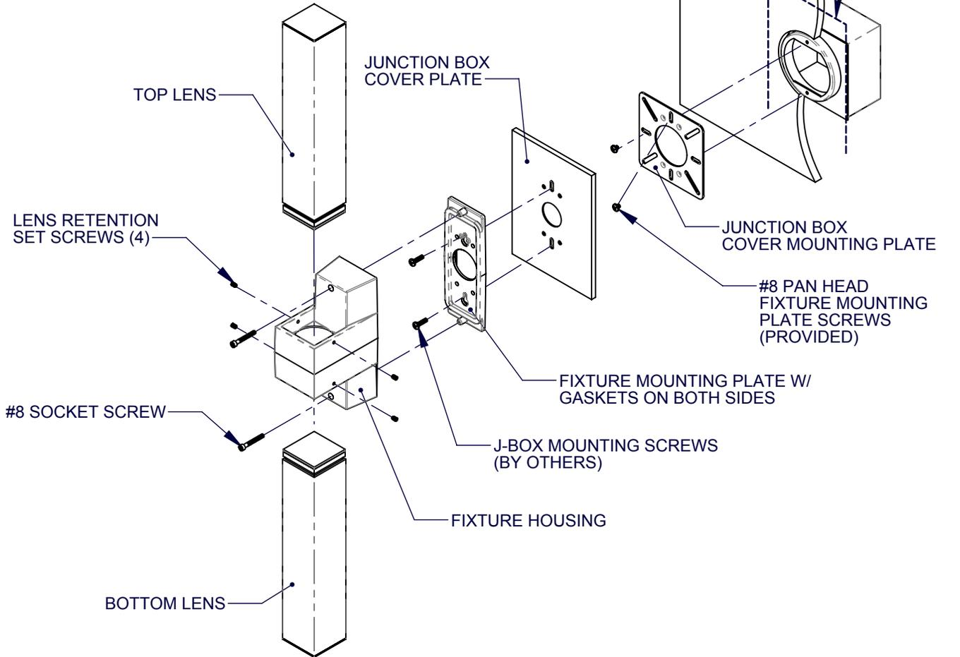
**Important:** Exterior installation requires caulk along perimeter of housing (or J-Box Cover). SEE SHEET 4.
