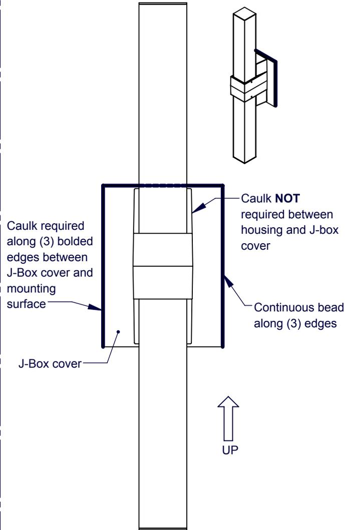
**IMPORTANT:** Caulk must be applied to a clean and dry surface. All surfaces must be free of debris and residue to ensure a watertight seal. Faulty or missing caulk will cause electronic failure.
