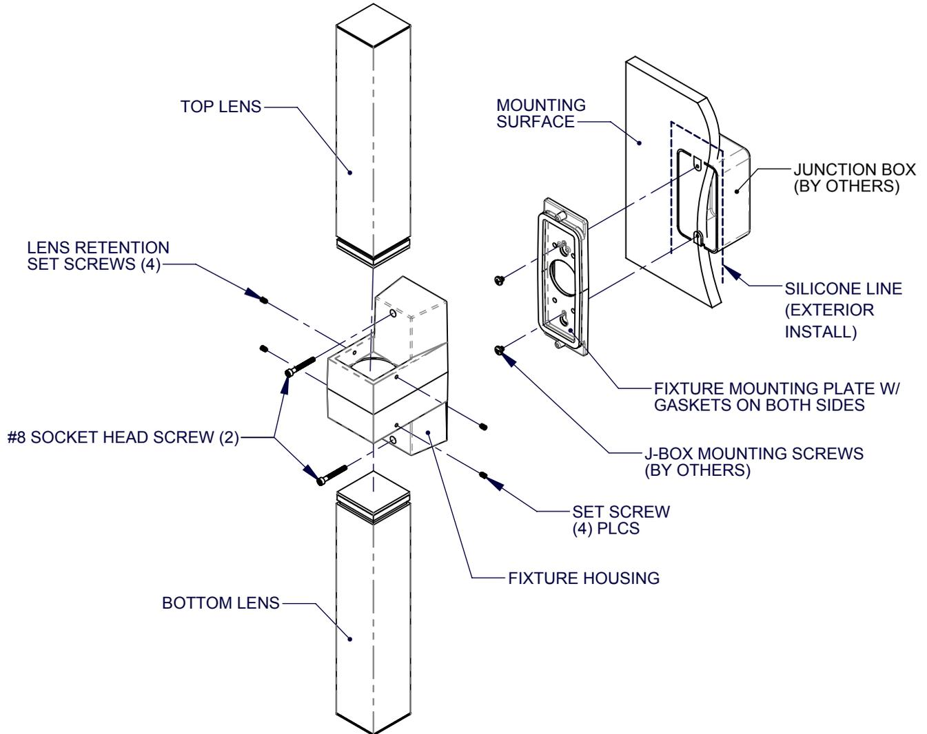
**Important:** Exterior installation requires caulk along perimeter of housing (or J-Box Cover). SEE SHEET 4.
