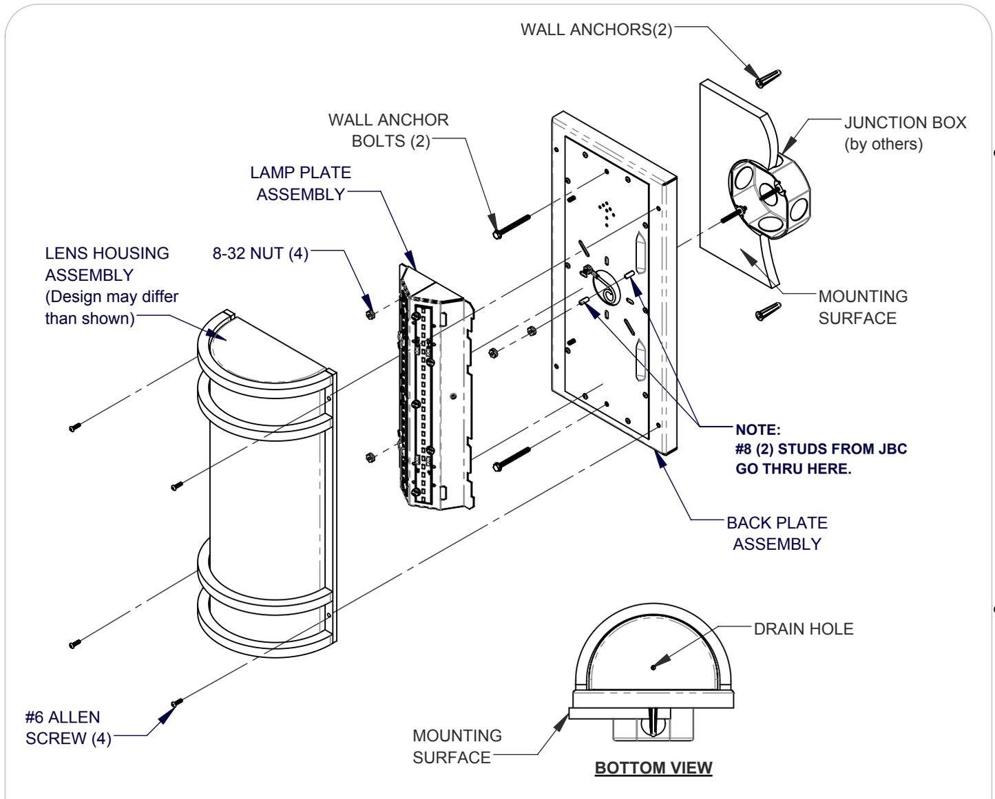
1. Thread the 1 1/2" #8 set screws into the junction box (by others). Leave about 1" of the set screws coming off of the junction box.
