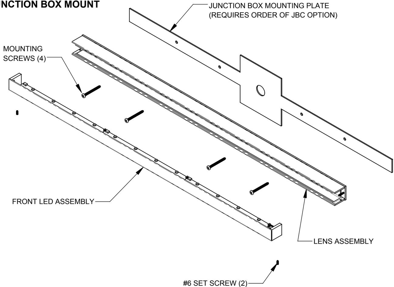
1. Mount junction box mounting plate (requires order of JBC option) to mounting surface, covering the junction box (by others).
